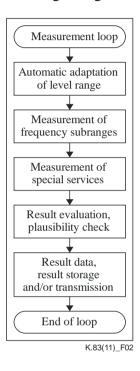
Figure 2 – Measurement loop
