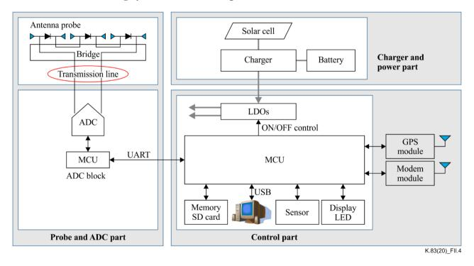
Figure II.4 – Broadband EMF area monitor block diagram
