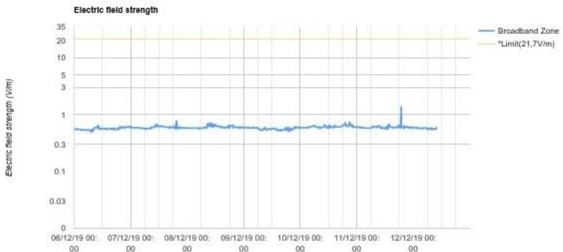
Figure II.17 – Results of the EMF measurement
