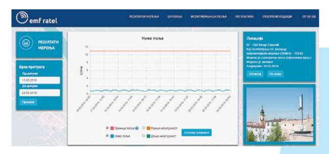
Figure 4. EM field levels for a sensor located at elementary school "Lazar Savatic" in Belgrade
