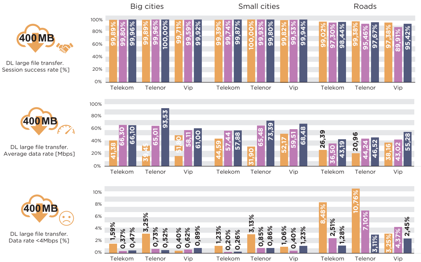
Figure 11.4. FDTT HTTP data transmission service testing results (DL 400MB)
