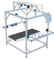
Identification systems with CLV, Matrix cameras Identification of shipments on Pre-sorter
