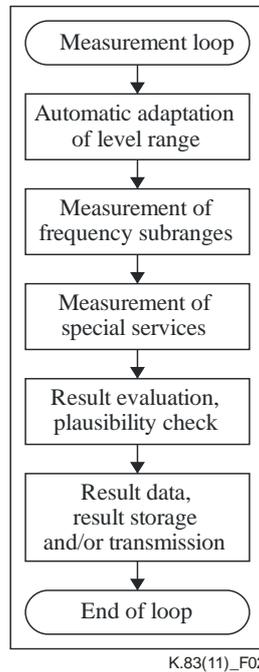
**Figure 2 – Measurement loop**
